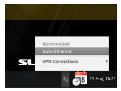
Once the network is enabled select "Auto Ethernet" if you have DHCP active. For wired connections, you will be ready to connect at this point. If you are using a wireless connection, return to the networking menu and select the correct SSID (wireless network).
