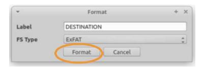
Verification of the formatting can be found in the Task Logs. Once the format is completed click the "Refresh" button in the Disk Manager to re-poll the devices to show the newly formatted volume.
