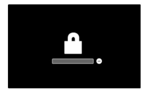
You must enter the Firmware Password PIN or passcode in order to see the boot options (this includes RECON IMAGER if it is attached).
