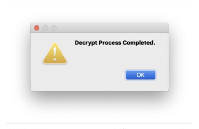
If the FileVault volume was on a macOS Extended file system (HFS+) a new decrypted volume will mount with a new disk number.
