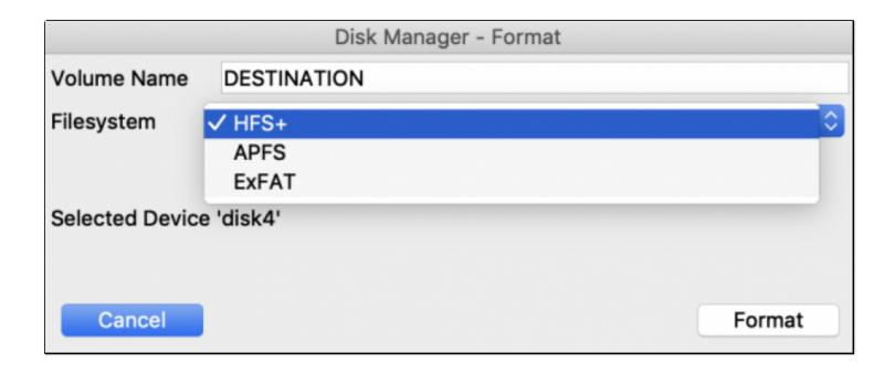
Once the collection drive has been formatted it is always good practice to attach the destination drive to the examination system to see if it will be detected properly. Although, the file system is correct the examination system may not recognize the partition scheme used in formatting. This is especially true of older operating systems.
