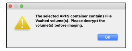
Once the partition is decrypted using the password, select the FileVault encrypted volume as a source in Disk Imager and click Refresh.
