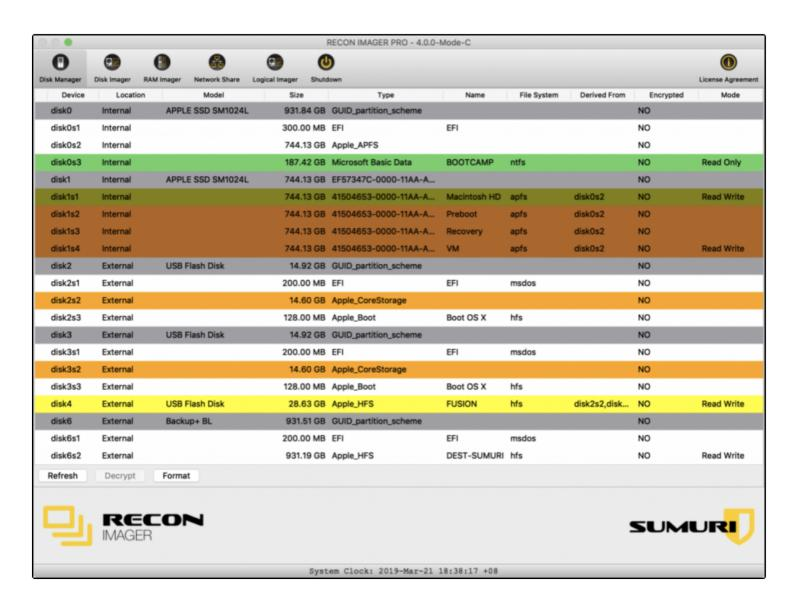
The Disk Manager allows you to see all connected devices to the Mac in a software write-blocked environment. Each system can vary, however, the Disk Manager will show all traditional, virtual or synthesized physical disks and logical volumes.
