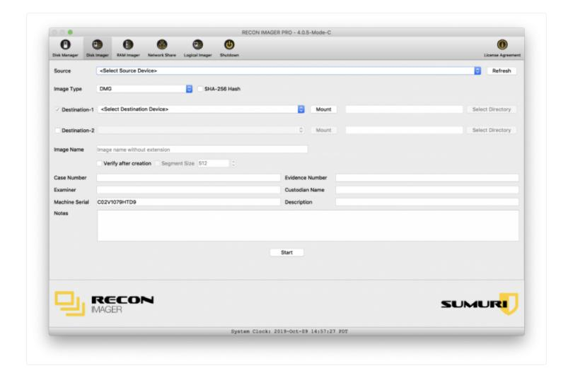
The RECON IMAGER Disk Imager allows for the acquisition of any internal disk(s) or volumes or any attached storage media including other Macs in Target Disk Mode. The options presented in the Disk Imager will change depending on what Image Type (output format) is selected.
